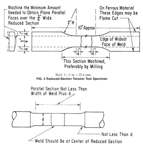
NOTE 1—The ends may be of any shape to fit the holders of the testing machine in such a way that the load is applied axially. FIG. 4 Alternative Reduced-Section Tension Test Specimen
